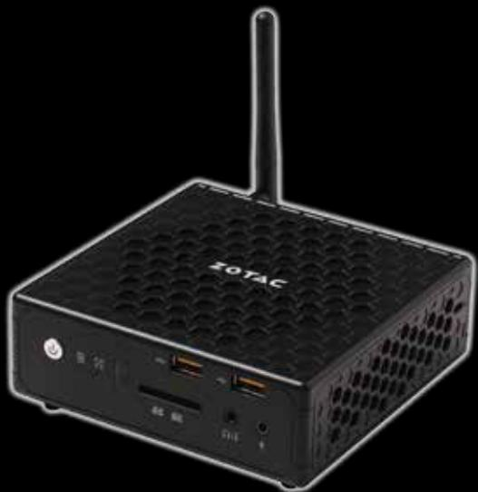
Enjoy quiet computing in a palm-sized form factor with the ZOTAC ZBOX CI320 nano series mini-PC. The ZOTAC ZBOX CI320 nano series mini-PC features a special passive-cooled chassis that eliminates cooling fans to create zero noise for a peaceful silent computing experience.
